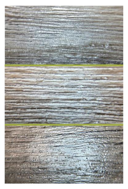
The above photos help illustrate the results of the Sim Floor Scratch Resistance tests. It's easy to see why the Ceramic Coating was rated a 3.5 - scratches are easily visible and there is a noticeable gloss difference where the wear tester made contact with the sample. However, both the NovaShield® Coating and the Diamond Coating showed no visible scratches and only a slight change in appearance.
