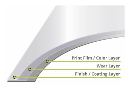
Most polyurethane coatings are reinforced with hard and very fine minerals, which are designed to improve the scratch resistance of the finish. However, the scratch resistance of these minerals varies and has a direct impact on the performance of the finish. As the hardness of minerals increases, so too does the inflexibility of
