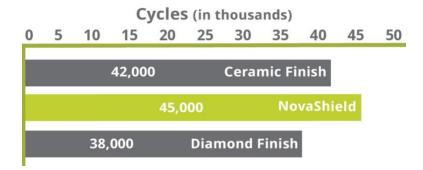
The way the diamond coating wore was also interesting - while it's normal for test samples to indent slightly and have a higher sheen in the wheel path, the diamond coating whitened, deteriorated and built up in the traffic pattern. This could be due to the inflexibility of the diamond mineral in the coating. Regardless, it
