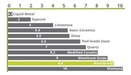
The proprietary mineral used within the NovaShield® finish has a Mohs rating of 9.4. When comparing NovaShield® to Modified Ceramic (8.2) and Aluminum Oxide (9), it may not seem like a significant difference in scratch resistance. However, since the Mohs scale is ordinal, NovaShield® is over twice as hard as Aluminum Oxide and nearly four times as hard as Modified Ceramics.
