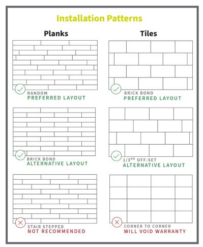
**Layout:** Prior to installation, confirm the installation pattern and direction per the design specifications or work order. Planks should be installed in a random pattern - plank end joints should be randomly spaced by  $\geq$  8-in. Avoid "H" joints and do not install in
