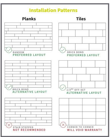
**Layout:** Prior to installation, confirm the installation pattern and direction per the design specifications or work order. Planks should be installed in a random pattern - plank end joints should be randomly spaced by  $\ge$  8-in. Avoid "H" joints and do not install in
